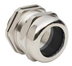
Bimed cable gland, PG42 thread type, nickel-plated brass, accepts 30 to 38mm diameter cable, IP68. Mounting hardware included.
