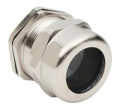
Bimed cable gland, PG36 thread type, nickel-plated brass, accepts 22 to 32mm diameter cable, IP68. Package of 2. Mounting hardware included.
