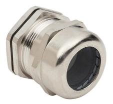
Bimed cable gland, PG29 thread type, nickel-plated brass, accepts 18 to 25mm diameter cable, IP68. Package of 5. Mounting hardware included.
