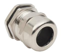
Bimed cable gland, PG21 thread type, nickel-plated brass, accepts 13 to 18mm diameter cable, IP68. Package of 5. Mounting hardware included.
