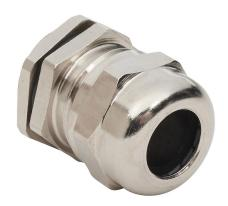
Bimed cable gland, PG13.5 thread type, nickel-plated brass, accepts 6 to 12mm diameter cable, IP68. Package of 5. Mounting hardware included.
