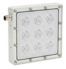
Lumher BS machine vision lighting, spot light, white light emission, 5000K, plus or minus 3 degrees, continuous, 125 x 125 x 25mm housing, 22.8-25.2 VDC operating voltage.
