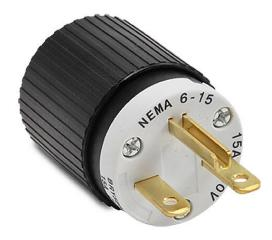
Bryant industrial heavy duty straight blade plug, 15A, 250 VAC, 1-phase, 2-pole, 3-wire, NEMA 6-15, accepts cord size 0.3-0.65in, nylon housing, black and white.
