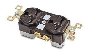
Bryant industrial heavy duty duplex straight blade receptacle, 15A, 250 VAC, 1-phase, 2-pole, 3-wire, NEMA 6-15, nylon molded housing, brown.
