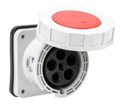
Bryant watertight single pin and sleeve receptacle, 60A, 277/480 VAC, 3-phase, 4-pole, 5-wire, 7 hour, IP67, nylon housing, red.
