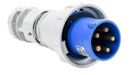
Bryant watertight pin and sleeve plug, 60A, 120/208 VAC, 3-phase, 4-pole, 5-wire, 9 hour, accepts cord size 1.18-1.45in, IP67, nylon housing, blue.
