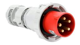
Bryant watertight pin and sleeve plug, 60A, 277/480 VAC, 3-phase, 4-pole, 5-wire, 7 hour, accepts cord size 1.18-1.45in, IP67, nylon housing, red.
