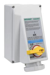
Bryant pin and sleeve mechanical interlock, rotary, enclosed, load break capable, 208Y/120 VAC, 60A, 3-phase, 4-pole, 5-wire, 9 hour pin and sleeve receptacle, 10kA SCCR, 11.9in x6.9in x8.6in housing.
