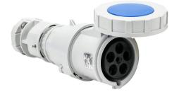
Bryant watertight pin and sleeve connector, 60A, 120/208 VAC, 3-phase, 4-pole, 5-wire, 9 hour, accepts cord size 1.18-1.45in, IP67, nylon housing, blue.
