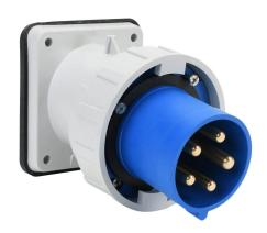
Bryant watertight pin and sleeve inlet, 60A, 120/208 VAC, 3-phase, 4-pole, 5-wire, 9 hour, IP67, nylon housing, blue.
