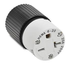
Bryant industrial heavy duty straight blade connector, 20A, 250 VAC, 1-phase, 2-pole, 3-wire, NEMA 6-20, accepts cord size 0.3-0.65in, nylon housing, black and white.
