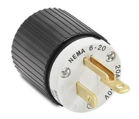
Bryant industrial heavy duty straight blade plug, 20A, 250 VAC, 1-phase, 2-pole, 3-wire, NEMA 6-20, accepts cord size 0.3-0.65in, nylon housing, black and white.
