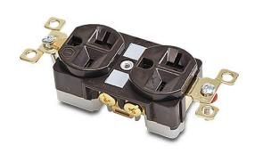
Bryant industrial heavy duty duplex straight blade receptacle, 20A, 250 VAC, 1-phase, 2-pole, 3-wire, NEMA 6-20, nylon molded housing, brown.
