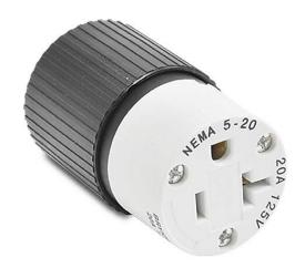
Bryant industrial heavy duty straight blade connector, 20A, 125 VAC, 1-phase, 2-pole, 3-wire, NEMA 5-20, accepts cord size 0.3-0.65in, nylon housing, black and white.
