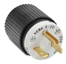
Bryant industrial heavy duty straight blade plug, 20A, 125 VAC, 1-phase, 2-pole, 3-wire, NEMA 5-20, accepts cord size 0.3-0.65in, nylon housing, black and white.
