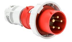
Bryant watertight pin and sleeve plug, 30A, 277/480VAC, 3-phase, 4-pole, 5-wire, 7 hour, accepts cord size 0.76-1.15in, IP67, nylon housing, red.
