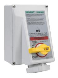
Bryant pin and sleeve mechanical interlock, rotary, enclosed, load break capable, 480Y/277 VAC, 30A, 3-phase, 4-pole, 5-wire, 7 hour pin and sleeve receptacle, 10kA SCCR, 10.1in x6.9in x7.8in housing.
