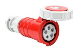
Bryant watertight pin and sleeve connector, 30A, 277/480VAC, 3-phase, 4-pole, 5-wire, 7 hour, accepts cord size 0.76-1.15in, IP67, nylon housing, red.
