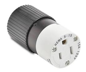
Bryant industrial heavy duty straight blade connector, 15A, 125 VAC, 1-phase, 2-pole, 3-wire, NEMA 5-15, accepts cord size 0.3-0.65in, nylon housing, black and white.
