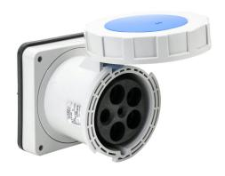
Bryant watertight single pin and sleeve receptacle, 100A, 120/208 VAC, 3-phase, 4-pole, 5-wire, 9 hour, IP67, nylon housing, blue.
