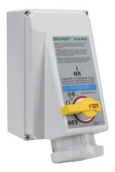
Bryant pin and sleeve mechanical interlock, rotary, enclosed, load break capable, 208Y/120 VAC, 100A, 3-phase, 4-pole, 5-wire, 9 hour pin and sleeve receptacle, 10kA SCCR, 11.9in x6.9in x9.3in housing.
