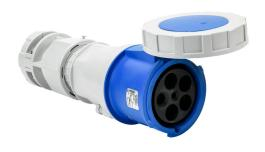
Bryant watertight pin and sleeve connector, 100A, 120/208 VAC, 3-phase, 4-pole, 5-wire, 9 hour, accepts cord size 1.063-1.88in, IP67, nylon housing, blue.
