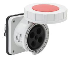
Bryant watertight single pin and sleeve receptacle, 60A, 480 VAC, 3-phase, 3-pole, 4-wire, 7 hour, IP67, nylon housing, red.
