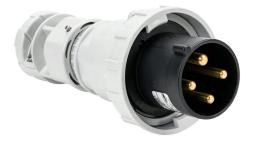
Bryant watertight pin and sleeve plug, 60A, 600 VAC, 3-phase, 3-pole, 4-wire, 5 hour, accepts cord size 1.05-1.45in, IP67, nylon housing, black.
