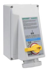
Bryant pin and sleeve mechanical interlock, rotary, enclosed, load break capable, 240 VAC, 60A, 3-phase, 3-pole, 4-wire, 9 hour pin and sleeve receptacle, 10kA SCCR, 11.9in x6.9in x8.6in housing.
