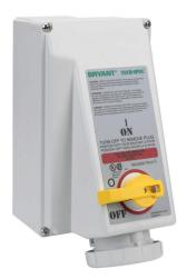
Bryant pin and sleeve mechanical interlock, rotary, enclosed, load break capable, 480 VAC, 60A, 3-phase, 3-pole, 4-wire, 7 hour pin and sleeve receptacle, 10kA SCCR, 11.9in x6.9in x8.6in housing.
