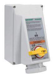
Bryant pin and sleeve mechanical interlock, rotary, enclosed, load break capable, 120/240 VAC, 60A, 1-phase, 3-pole, 4-wire, 12 hour pin and sleeve receptacle, 10kA SCCR, 11.9in x6.9in x8.6in housing.
