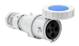
Bryant watertight pin and sleeve connector, 60A, 250 VAC, 3-phase, 3-pole, 4-wire, 9 hour, accepts cord size 1.05-1.45in, IP67, nylon housing, blue.
