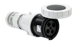
Bryant watertight pin and sleeve connector, 60A, 600 VAC, 3-phase, 3-pole, 4-wire, 5 hour, accepts cord size 1.05-1.45in, IP67, nylon housing, black.
