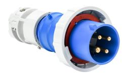
Bryant watertight pin and sleeve plug, 30A, 250 VAC, 3-phase, 3-pole, 4-wire, 9 hour, accepts cord size 0.625-1.05in, IP67, nylon housing, blue.
