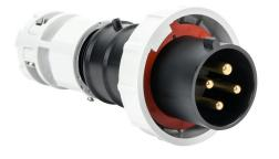
Bryant watertight pin and sleeve plug, 30A, 600 VAC, 3-phase, 3-pole, 4-wire, 5 hour, accepts cord size 0.625-1.05in, IP67, nylon housing, black.
