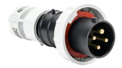
Bryant watertight pin and sleeve plug, 30A, 600 VAC, 3-phase, 3-pole, 4-wire, 5 hour, accepts cord size 0.625-1.05in, IP67, nylon housing, black.
