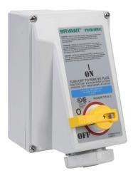
Bryant pin and sleeve mechanical interlock, rotary, enclosed, load break capable, 240 VAC, 30A, 3-phase, 3-pole, 4-wire, 9 hour pin and sleeve receptacle, 10kA SCCR, 10.1in x6.9in x7.8in housing.
