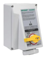
Bryant pin and sleeve mechanical interlock, rotary, enclosed, load break capable, 600 VAC, 30A, 3-phase, 3-pole, 4-wire, 5 hour pin and sleeve receptacle, 10kA SCCR, 10.1in x6.9in x7.8in housing.
