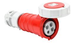
Bryant watertight pin and sleeve connector, 30A, 480 VAC, 3-phase, 3-pole, 4-wire, 7 hour, accepts cord size 0.625-1.05in, IP67, nylon housing, red.
