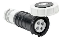
Bryant watertight pin and sleeve connector, 30A, 600 VAC, 3-phase, 3-pole, 4-wire, 5 hour, accepts cord size 0.625-1.05in, IP67, nylon housing, black.
