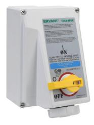
Bryant pin and sleeve mechanical interlock, rotary, enclosed, load break capable, 240 VAC, 20A, 3-phase, 3-pole, 4-wire, 9 hour pin and sleeve receptacle, 10kA SCCR, 10.1in x6.9in x7.8in housing.
