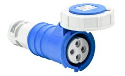
Bryant watertight pin and sleeve connector, 20A, 250 VAC, 3-phase, 3-pole, 4-wire, 9 hour, accepts cord size 0.41-0.65in, IP67, nylon housing, blue.
