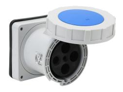
Bryant watertight single pin and sleeve receptacle, 100A, 250 VAC, 3-phase, 3-pole, 4-wire, 9 hour, IP67, nylon housing, blue.
