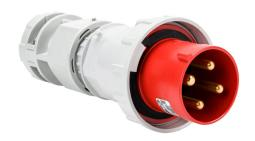
Bryant watertight pin and sleeve plug, 100A, 480 VAC, 3-phase, 3-pole, 4-wire, 7 hour, accepts cord size 0.905-1.68in, IP67, nylon housing, red.
