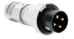
Bryant watertight pin and sleeve plug, 100A, 600 VAC, 3-phase, 3-pole, 4-wire, 5 hour, accepts cord size 0.905-1.68in, IP67, nylon housing, black.
