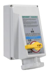
Bryant pin and sleeve mechanical interlock, rotary, enclosed, load break capable, 240 VAC, 100A, 3-phase, 3-pole, 4-wire, 9 hour pin and sleeve receptacle, 10kA SCCR, 11.9in x6.9in x9.3in housing.
