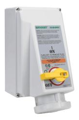
Bryant pin and sleeve mechanical interlock, rotary, enclosed, load break capable, 120/240 VAC, 100A, 1-phase, 3-pole, 4-wire, 12 hour pin and sleeve receptacle, 10kA SCCR, 11.9in x6.9in x9.3in housing.
