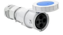
Bryant watertight pin and sleeve connector, 100A, 250 VAC, 3-phase, 3-pole, 4-wire, 9 hour, accepts cord size 0.905-1.68in, IP67, nylon housing, blue.
