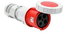
Bryant watertight pin and sleeve connector, 100A, 480 VAC, 3-phase, 3-pole, 4-wire, 7 hour, accepts cord size 0.905-1.68in, IP67, nylon housing, red.
