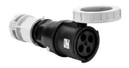
Bryant watertight pin and sleeve connector, 100A, 600 VAC, 3-phase, 3-pole, 4-wire, 5 hour, accepts cord size 0.905-1.68in, IP67, nylon housing, black.
