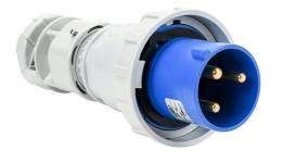
Bryant watertight pin and sleeve plug, 60A, 250 VAC, 1-phase, 2-pole, 3-wire, 6 hour, accepts cord size 0.97-1.45in, IP67, nylon housing, blue.
